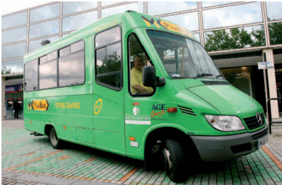
UV Modular Treka bodied Mercedes-Benz Sprinters are used on MK PlusBus services.
